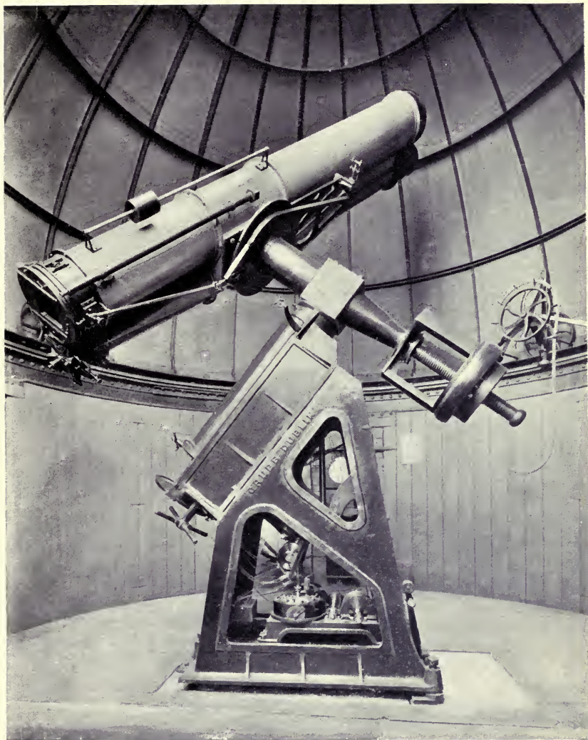
The 'Astrographic Telescope' of the Royal Observatory, Greenwich, i.e. the Photographic Telescope in use for the International Photographic Chart of the Heavens.
