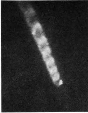
Figure 2.4. A glowing beam of electrons spirals upwards along the earth's magnetic field. This television image was taken during the Echo 7 sounding-rocket experiment. The view shows a portion of the corkscrew beam several hundred meters long from top to bottom and 17 meters across. The small, bright glow at the lower end of the beams is the accelerator that produced the energetic particles (courtesy John R. Winckler, University of Minnesota).
