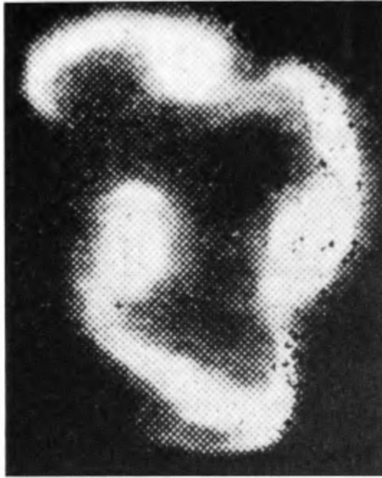
Figure 2.23. Cross-sectional view of a 2.1 mA electron beam.
